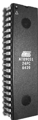
(c)DIP 封装 AT89C51
